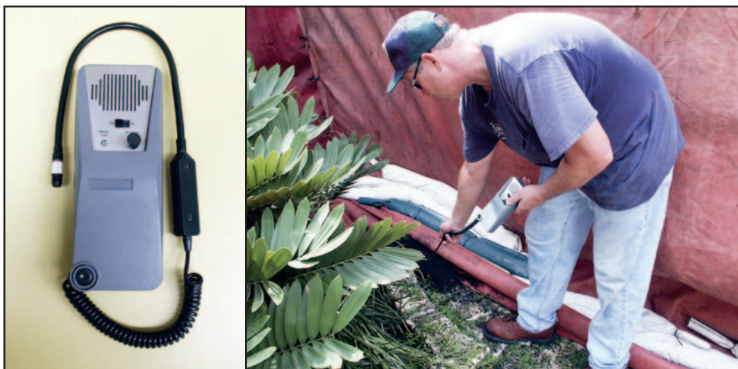
Figure 7-7. Tif halogen gas leak detector (left) being used to locate leaks (right) so they can be sealed.
