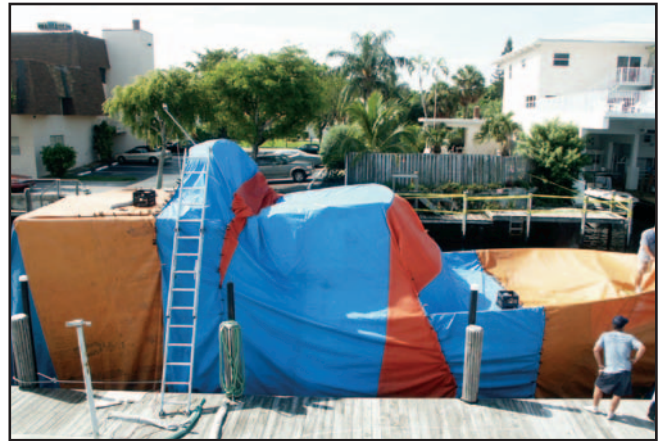
Figure 10-14. Note the depression on the bow created by the railings in the boat at right. Provisions for storm runoff were made using a PVC pipe drain leading to a side seam.
