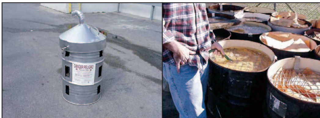
Figure 11-14. Deactivation of spent metallic phosphide. Dry (left) and wet methods (right). Photos courtesy of Degesch America.
