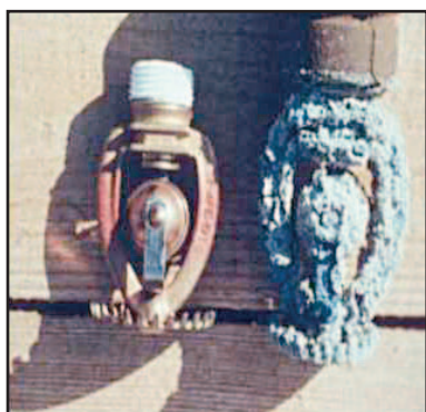
Figure 11-9. Corrosion of copper alloy (brass) fixtures due to high humidity, warm temperatures, and phosphine concentrations above 100 ppm. Photo courtesy of Degesch America.
