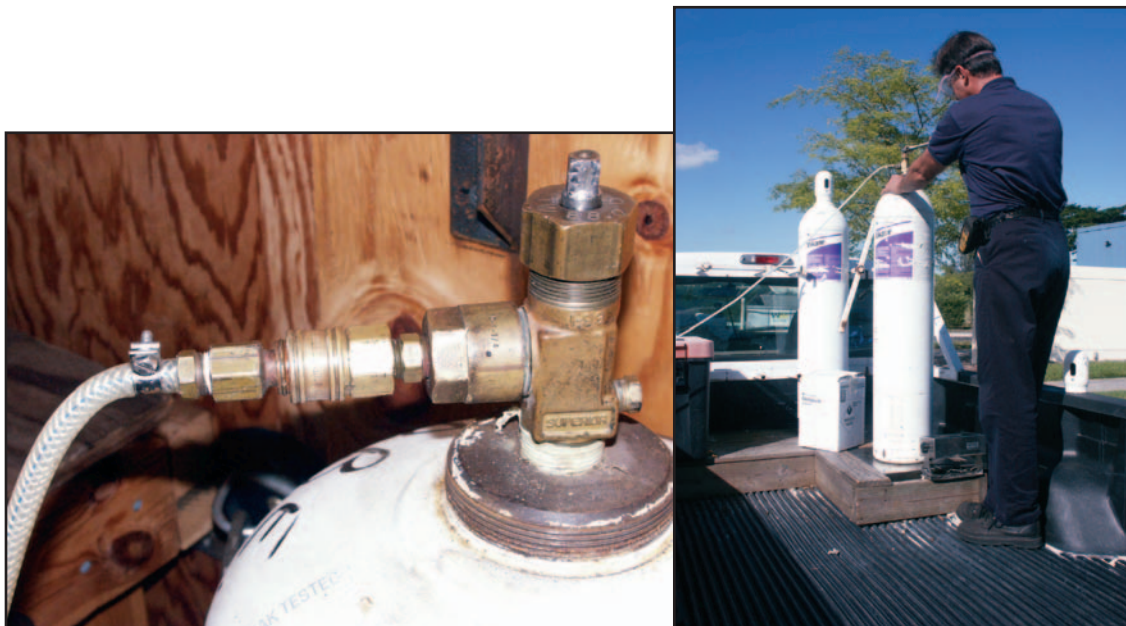
Figure 7-6. Hose clamp and hose adapter assembly (left). SF being released into structure (right).
