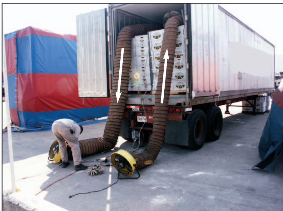
Figure 11-7. Active aeration proceeds by forcing air into container with one fan and pulling air out with a second fan. Note that boxes under container continue to aerate passively.
