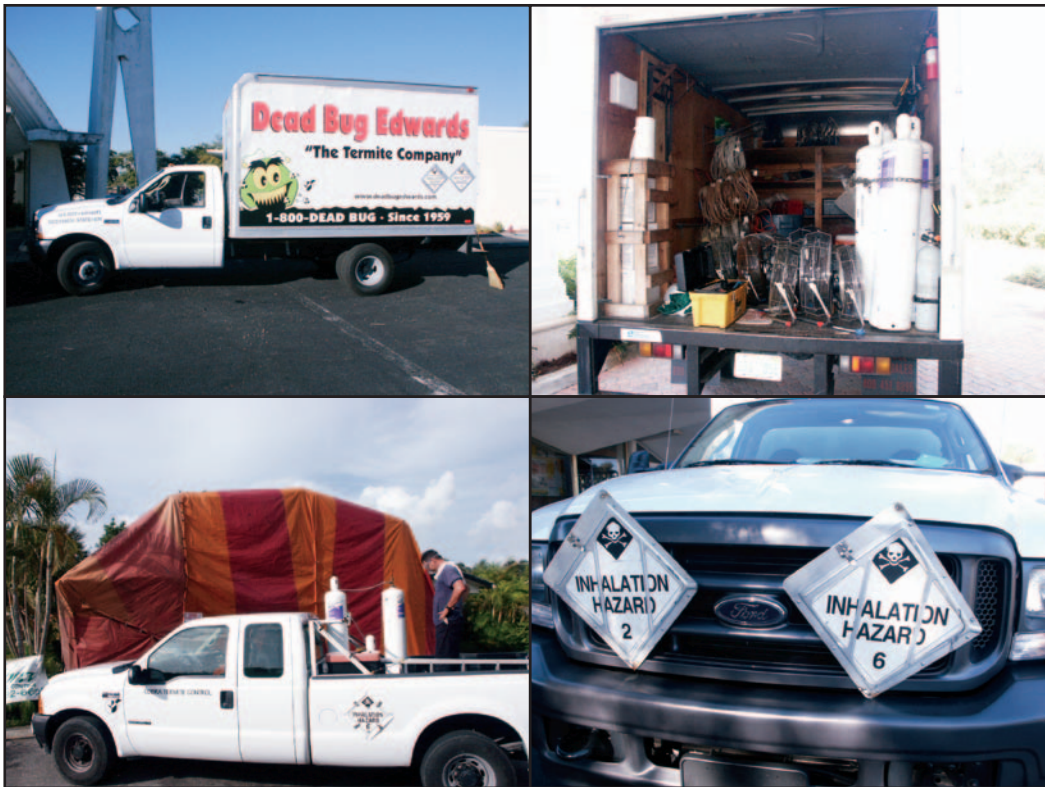
Figure 4-2. “Shooting” vehicles. Enclosed storage compartment (top). Open-air storage compartment and placarding (bottom). Note that driving compartments must be separated from SF storage. Note: Incorrect placard holder position. Holders should be turned and remounted by 90 degrees (bottom right).
