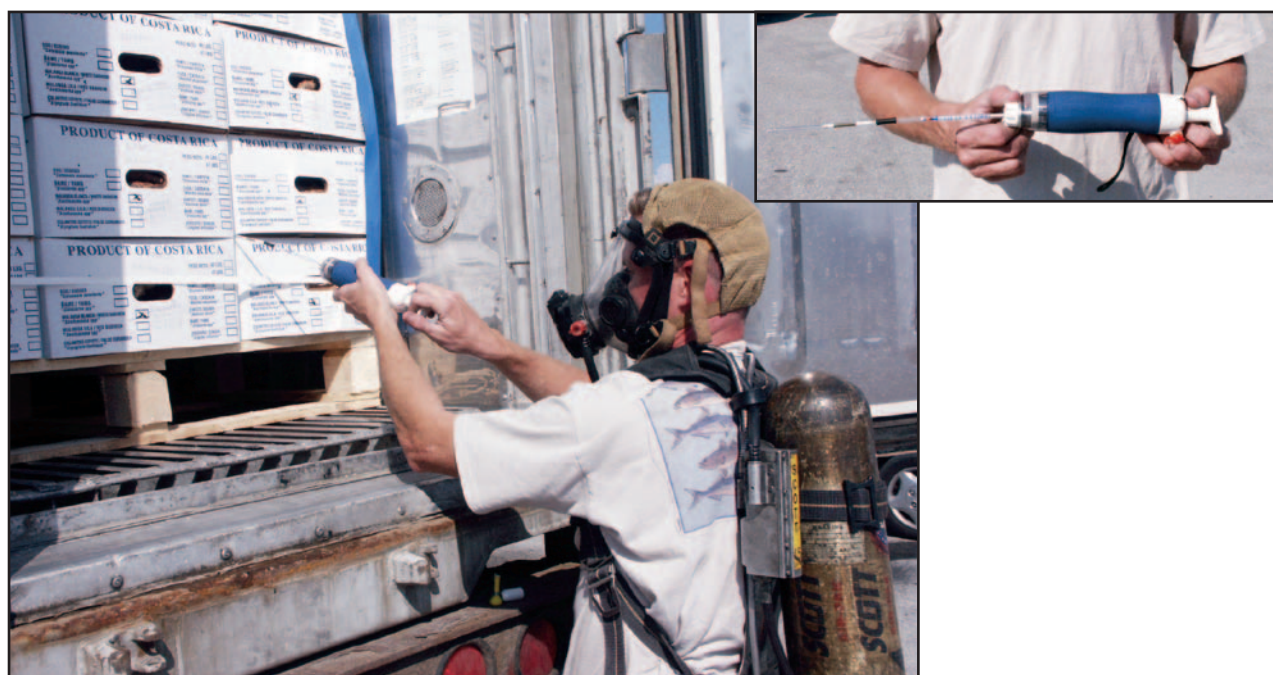
Figure 11-8. The commodity is cleared for release after 5 ppm or less MB is detected. The SPID, wearing an SCBA, is using a Kitagawa tube and pump apparatus (top right).
