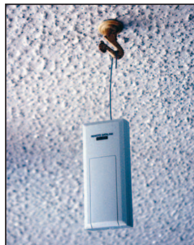
Figure 7-3. A weather station can measure temperature inside a fumigated building (left) using a wireless sensor(s) (right).
