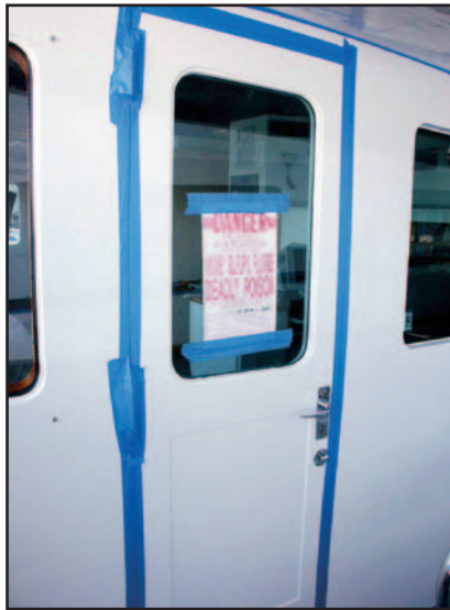
Figure 10-12. Here, 4-mil polyethylene sheeting and nonresidue masking tape is used for a gas-tight seal on a 153-ft. boat.
