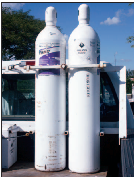
Figure 4-5. Exterior transport of sulfuryl fluoride. Vikane® cylinders must be upright, rigidly secured and with protective bonnets and valve covers attached. Note that the bottom bracket is missing and should be used.
