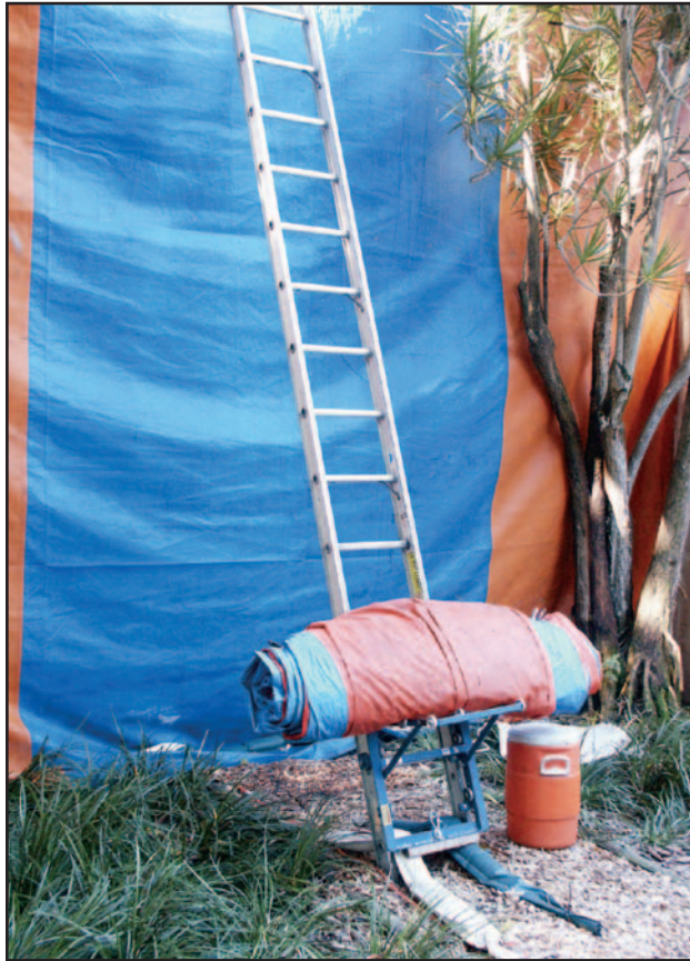
Figure 6-17. A ladder lift can safely elevate tarpaulins onto a roof (left). Balance and coordination are vital to carry tarps up a ladder (top right). Tarps are dropped down from roof (bottom right).
