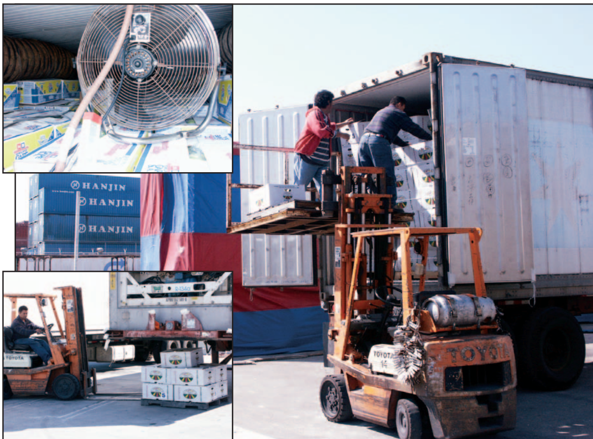
Figure 11-2. Fruit boxes are removed from the top of the container (trailer) to form a 2-ft headspace to aid in MB circulation (right). MB shooting fan and shooting hose in the container headspace (top left). Boxes from headspace are placed under the same container from which they were removed (bottom left).
