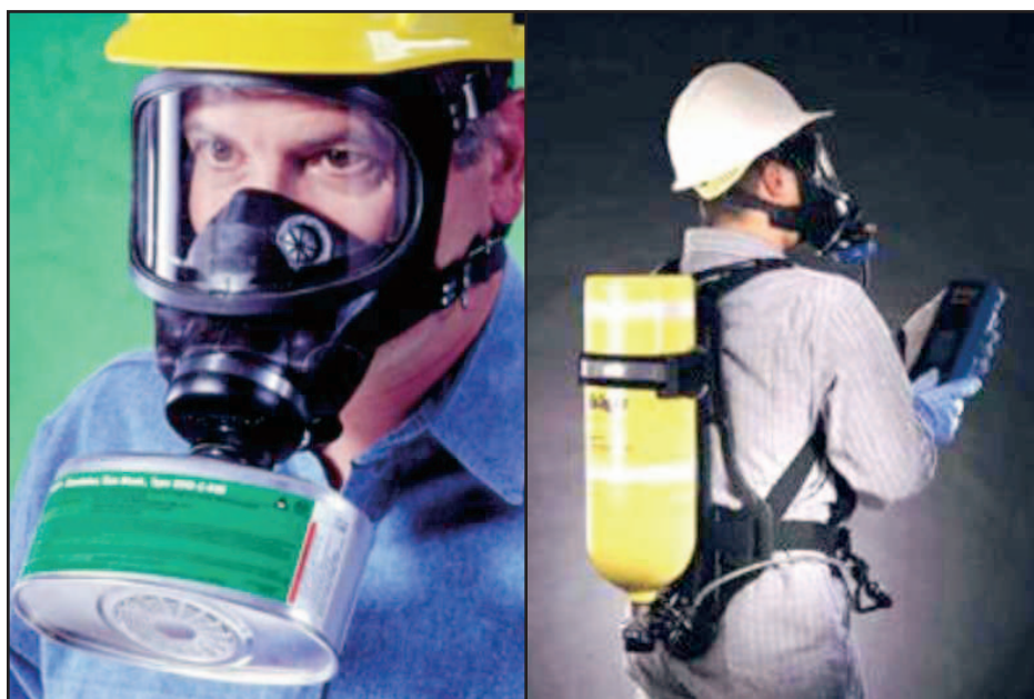
Figure 11-11. A canister gas mask with full face shield can be used in phosphine concentrations between 0.3-15 ppm (left). Above 15 ppm or if concentration is unknown, a SCBA is required (right). Photo courtesy of Degesch America.
