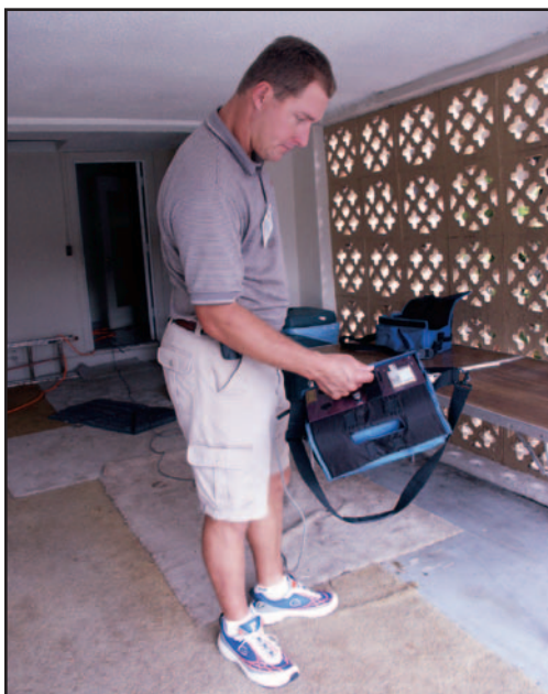
Figure 9-6. Interscan connected to wall outlet (note protective carrying case) (left). Interscan gas analyzer with portable battery pack (right).
