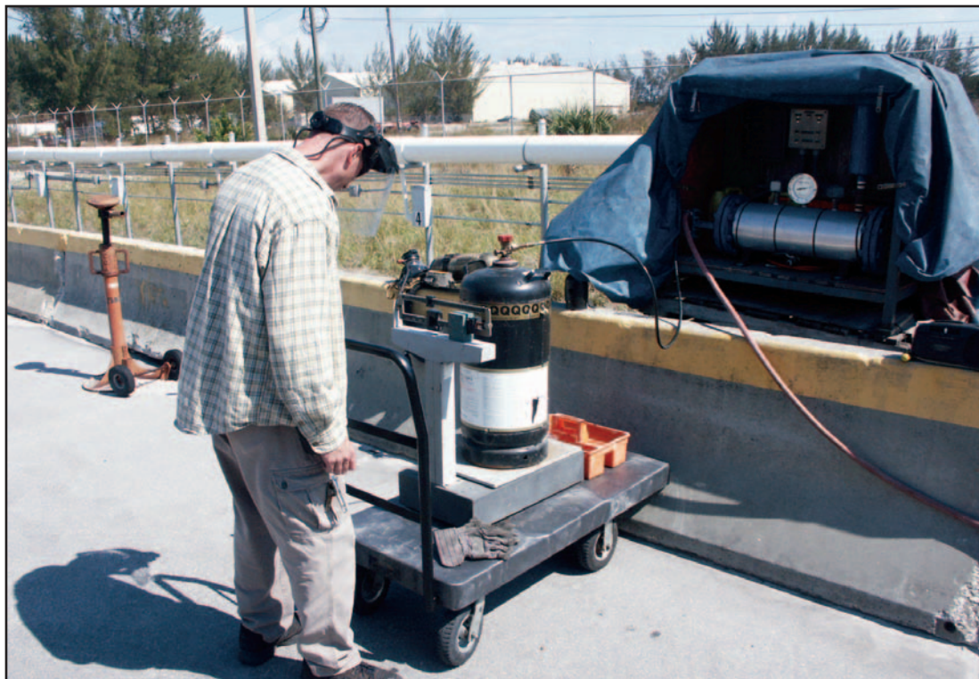
Figure 11-4. Methyl bromide is introduced into the commodity container in Fig 11-3. A 100-lb. cylinder of 100% MB is resting on a top loading scale that has been adjusted to read the desired weight loss. MB flows from the open valve into a heat exchanger (upper right) that converts the liquid into a hot gas ( >130^{\circ}\text{F} ) exiting through the heat resistant red shooting hose. Note the SPID is wearing a full face shield, long-sleeve shirt, long pants, socks and shoes, but no gloves.
