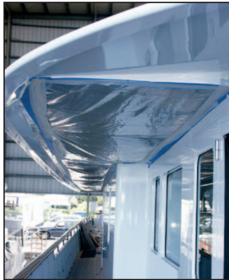
Figure 10-12. Here, 4-mil polyethylene sheeting and nonresidue masking tape is used for a gas-tight seal on a 153-ft. boat.
