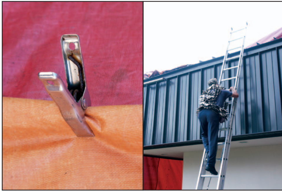
Figure 6-20. Fumigation clamp holding tarpaulin seam. Transporting clamps en masse on rope loops.
