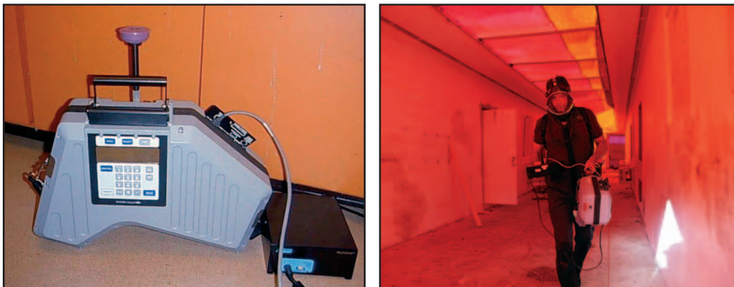
Figure 9-7. Miran infrared gas analyzer (left). In use (right).
