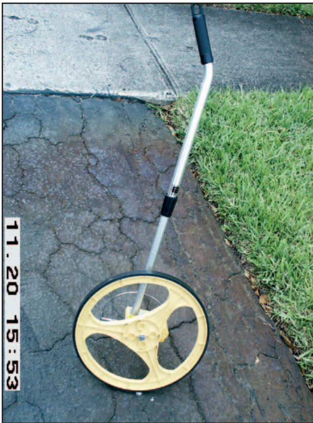
Figure 5-2. A measuring wheel allows for quick and accurate measurements on the ground or a flat roof. Measure the perimeter of a structure from where the tarp will drop.
