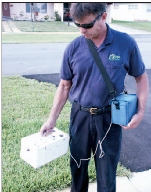
Figure 9-6. Interscan connected to wall outlet (note protective carrying case) (left). Interscan gas analyzer with portable battery pack (right).
