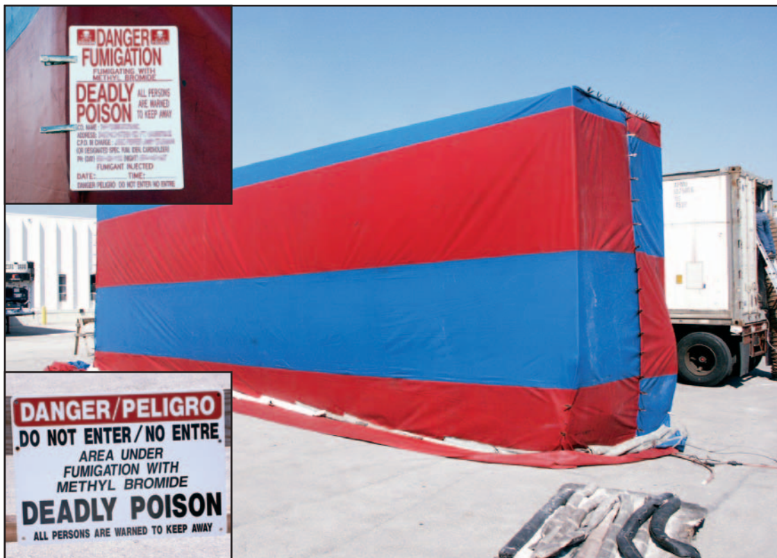
Figure 11-3. The container is tarped, snaked, and clamped as in a typical structural fumigation. Some containers can be taped and sealed, requiring a separate fumigation for the boxes removed from the headspace. The fumigation is conducted in a secure location marked with warning signs on the container (top left) and around the secured area (bottom left).
