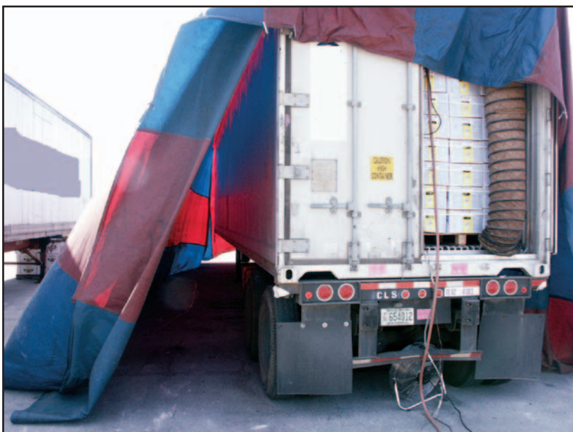
Figure 11-6. Passive aeration proceeds by removing clamps and snakes. The tarpaulin is removed a few minutes later.
