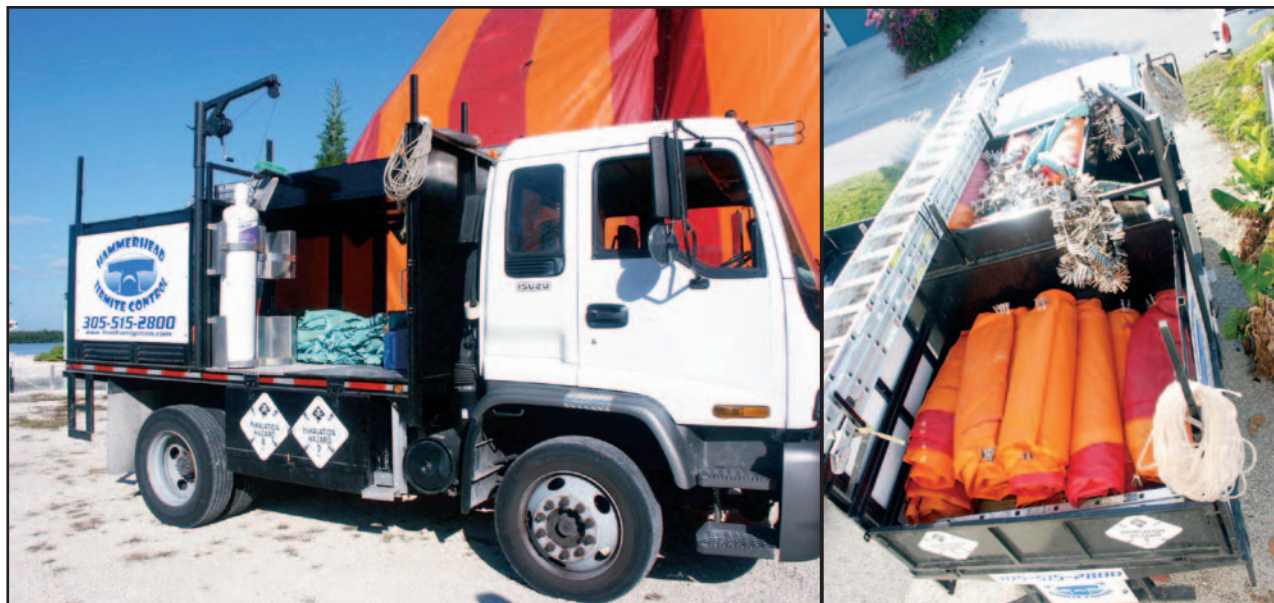
Figure 4-3. Combination vehicle for hauling both sealing and shooting equipment. Photos: M. Weinberg.
