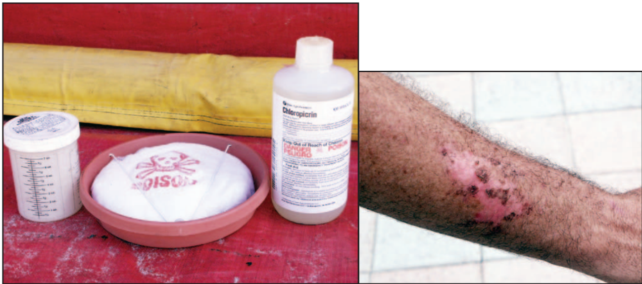
Figure 7-4. Graduated container with lid, evaporation pan, and chloropicrin bottle (left). Chloropicrin burn on forearm (right).
