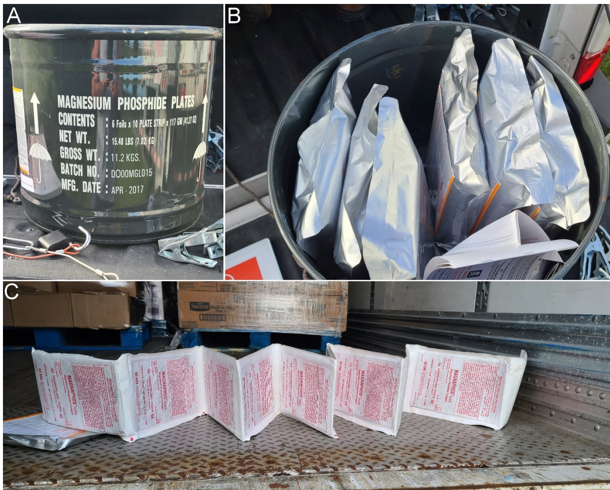
Figure 4-2. Packaging for magnesium phosphide plates. A: metal container with B: sealed sets of plates. C: exposed plates. (Photos: S. Brantley)
