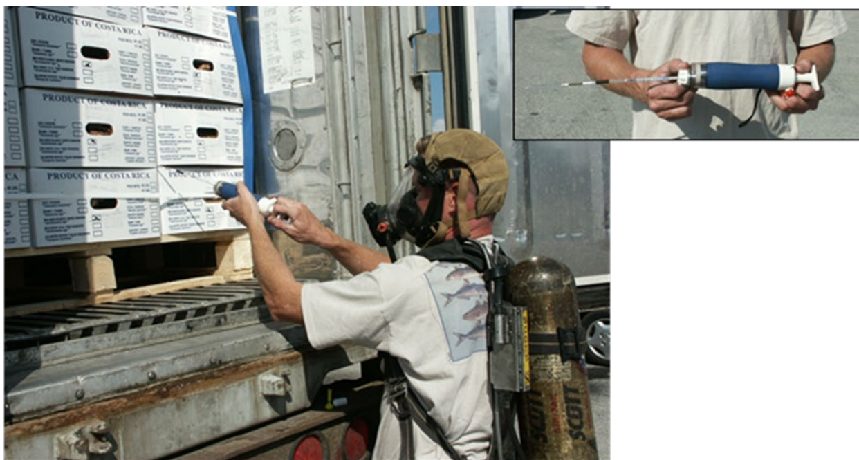
Figure 6-3. The fumigator, wearing a self-contained breathing apparatus (SCBA), is using a color diffusion detector tube connected to a pump apparatus to determine if the concentration of methyl bromide is 5 ppm or less after aeration of a fumigated commodity. (Photos: R. Scheffrahn)
