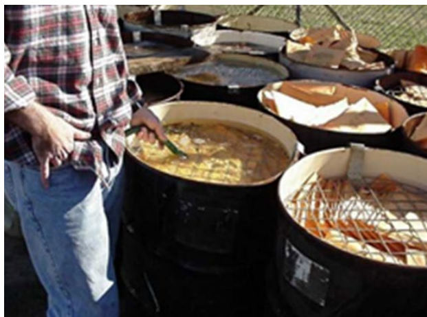
Figure 5-5. Deactivation of spent metallic phosphide. Wet (left) and dry methods (right). (Photos: Degesch America)
