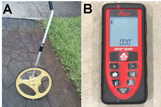
Figure 9-2. A: a measuring wheel allows for quick and accurate measurements from the ground or a flat roof. For tarped structures, measure the perimeter of a structure from where the tarp will drop. B: a laser distance meter is a convenient tool for measuring vertical heights and horizontal distances. (Photos: R. Scheffrahn, R. Borja)
