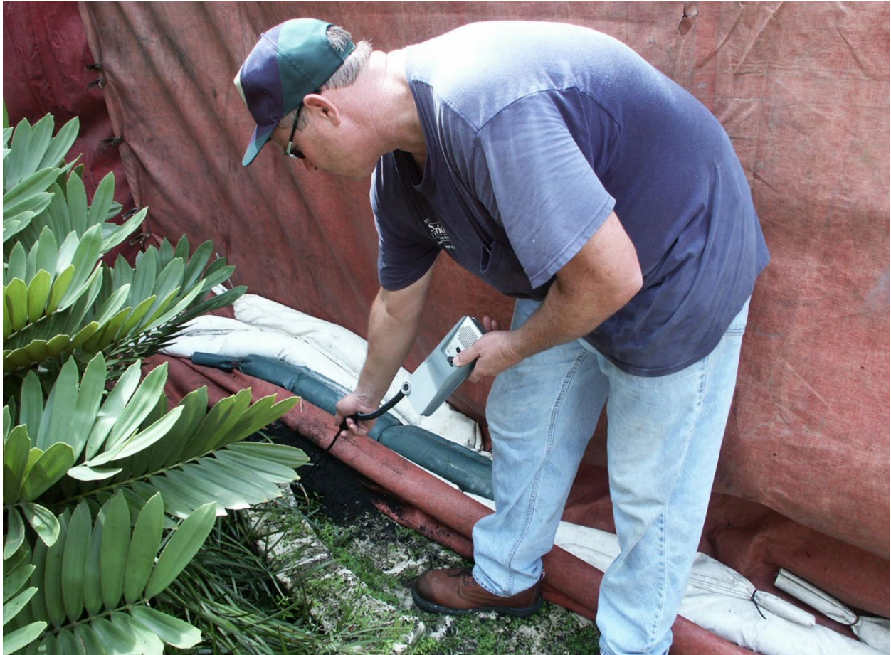
Figure 6-4. Use of a “leak detector” to determine if additional sealing is necessary. (Photo: R. Scheffrahn)
