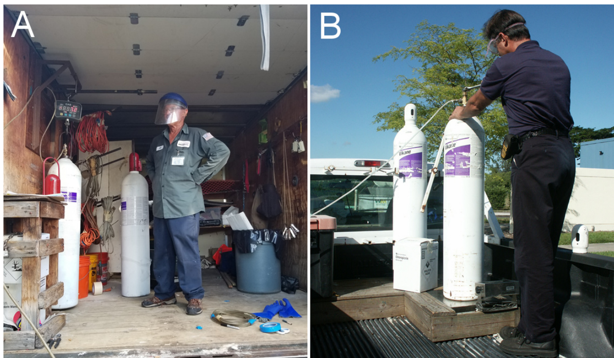
Figure 13-4. A: the fumigator is weighing an SF cylinder fitted with a hanging bonnet hooked to a hanging scale and is wearing a full face shield for eye protection. B: the fumigator is weighing a SF cylinder on top of a flatbed scale during fumigant introduction, is wearing safety goggles for eye protection. No gloves are worn. (Photos: T. Chouvenec, R. Scheffrahn)
