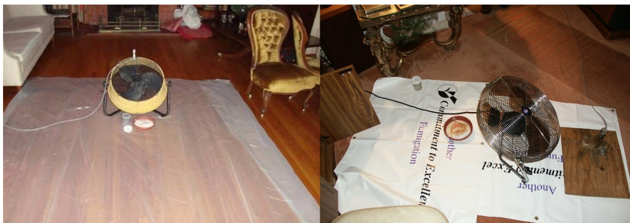
Figure 11-4. Chloropicrin pan and SF introduction fan with hose attached and all placed on polyethylene sheeting in a large, open space. (Photos: Douglas Products)
