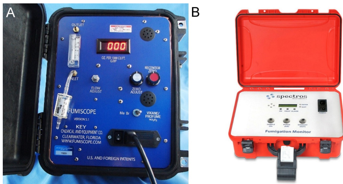
Figure 14-1. A: Fumiscope (Key Chemical and Equipment Co.) used to measure high concentrations (greater than 0.5 oz/1000 ft 3 ) of sulfuryl fluoride or methyl bromide. B: SF-ReportIR (Spectros Instruments) used to measure high concentrations (greater than 0.1 oz/1000 ft 3 ) of sulfuryl fluoride. (Photos: Key Chemical and Equipment Co, Spectros Instruments)
