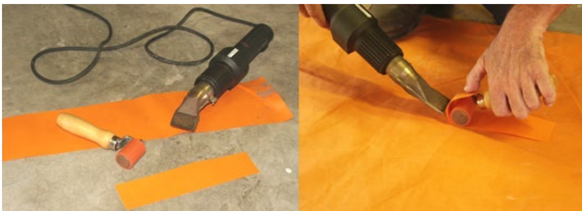
Figure 10-8. A heat patching kit can be used at the company site to repair damaged tarpaulins. (Photos: M. Weinberg)
