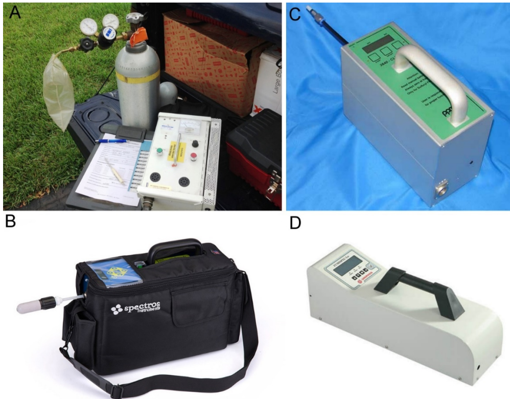
Figure 6-1. Approved low concentration detection (e.g., clearance) devices for sulfuryl fluoride fumigants, used to confirm a sulfuryl fluoride concentration of 1 ppm or less. A: Interscan (Interscan Corporation) and low ppm SF cylinder required to conduct calibration of the Interscan. B: SF-ExplorIR (Spectros Instruments). C: CLIRcheck (Cardinal Professional Products). D: FumiSpec Lo (Uniphos Envirotronic). (Photos: respective companies)
