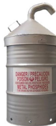
Figure 5-5. Deactivation of spent metallic phosphide. Wet (left) and dry methods (right). (Photos: Degesch America)
