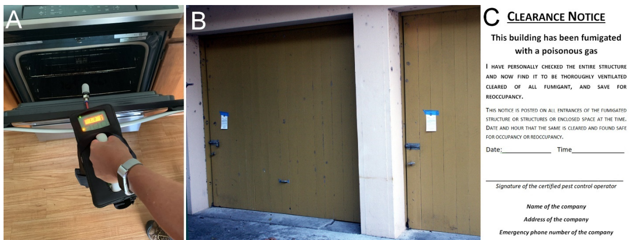
Figure 15-2. A: using a CLIRcheck to test for clearance of sulfuryl fluoride to 1 ppm or less in an oven that remained closed during the fumigation and aeration. B: after the structure is cleared, clearance notices are posted at each entryway. C: example of a clearance notice. (Photos: Douglas Products, R. Scheffrahn)
