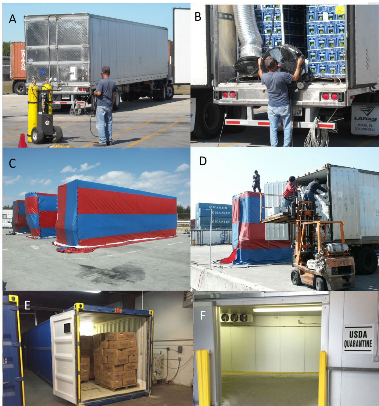
Figure 10-12. Plant Protection and Quarantine fumigations with MB. A: tarpless trailer fumigation in progress and B: tarpless fumigation following aeration. C: tarped shipping container fumigation and D: container fumigation following aeration. E: forty foot PPQ fumigation chamber. F. storage refrigerator after PPQ chamber produce is cleared. (Photos: R. Scheffrahn, Magic Fumigation)
