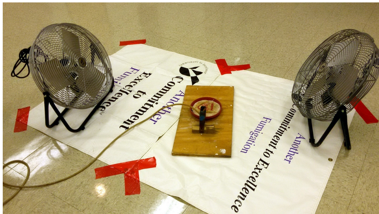
Figure 4-4. "Pic-pan". Shallow container with wicking material placed in the air stream of a fan, for the chloropicrin introduction. (Photo: T. Chouvinc)
