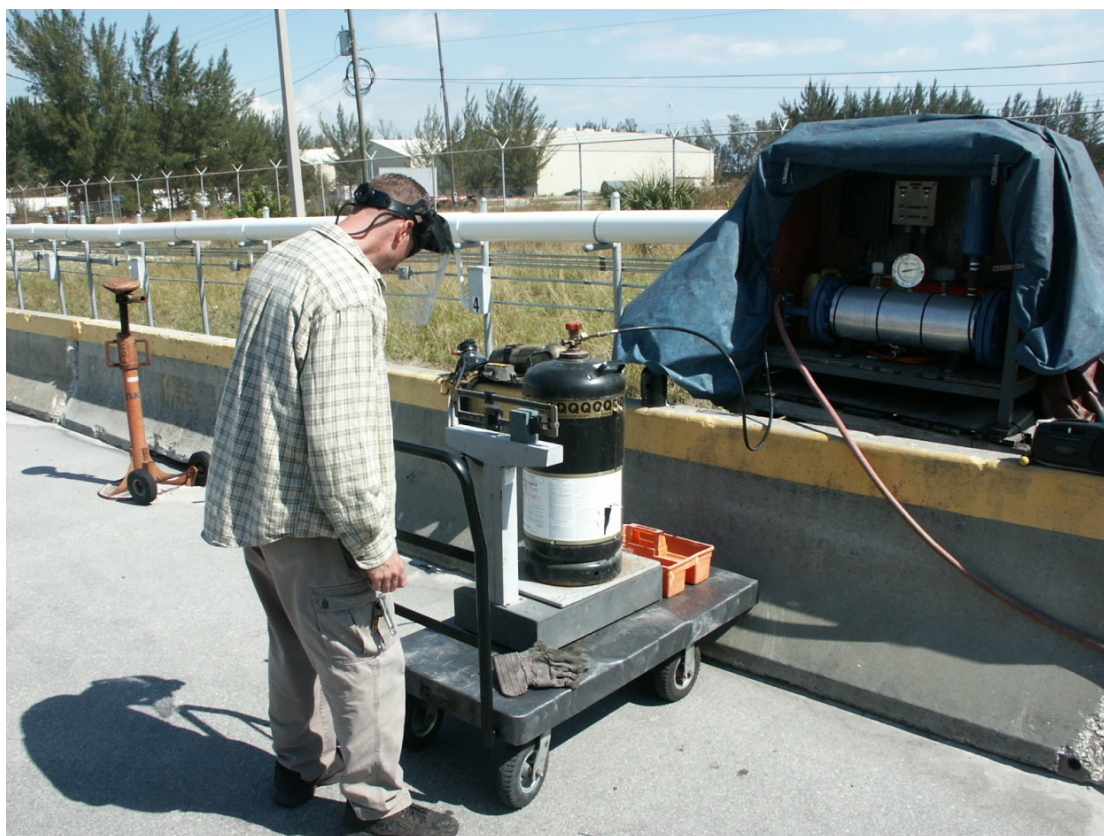
Figure 13-5. Methyl bromide is introduced into a commodity container for quarantine treatment. A 100-lb. cylinder of MB is resting on a flatbed scale that has been adjusted to read the desired weight loss. Methyl bromide flows from the open valve into a heat exchanger (upper right) that converts the liquid into a hot gas exiting through the heat resistant red shooting hose. Note that the fumigator is wearing a full face shield, long-sleeve shirt, long pants, shoes, and socks, while gloves are not worn. (Photo: R. Scheffrahn)
