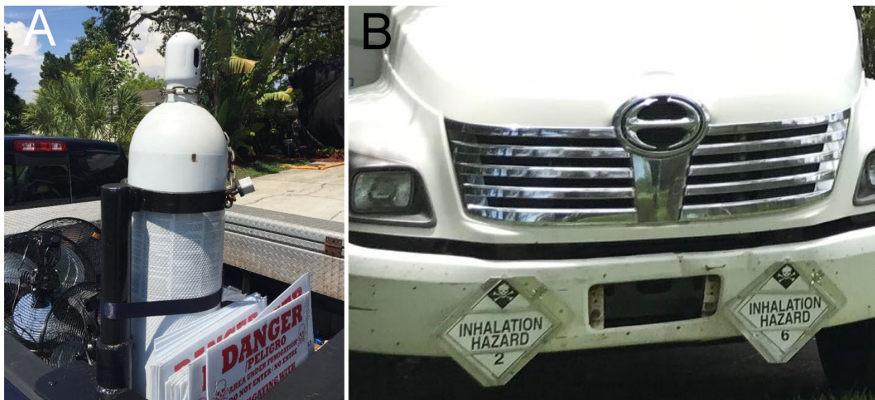
Figure 5-6. A: vehicle transport of sulfuryl fluoride cylinder; secure and upright, in separate airspace from vehicle occupants, and with valve cover and bonnet attached. B: placarding of vehicle transporting sulfuryl fluoride and chloropicrin; INHALATION HAZARD 2 (sulfuryl fluoride) placard (left) and the INHALATION HAZARD 6 (chloropicrin) placard (right). (Photos: Douglas Products)
